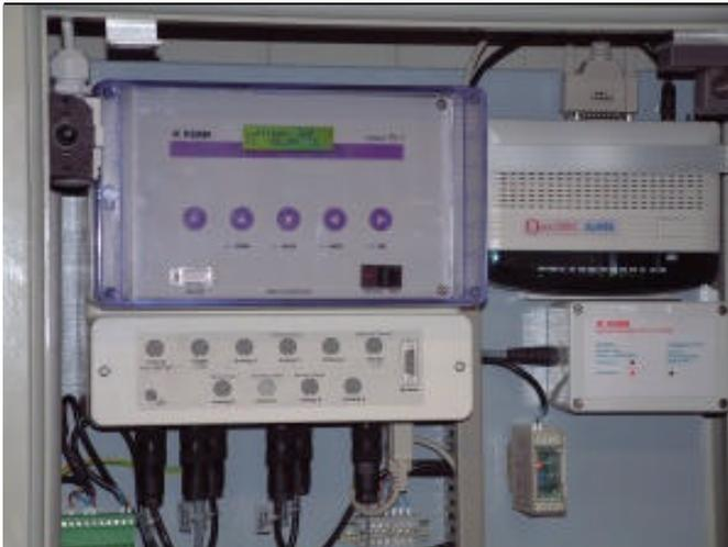
The Telelog TL-1 is a net- or solar powered data logger; its measuring networks can be build up to continually register and monitor any measuring values you like. The data interrogation can be made through the modem from different users at any time.
